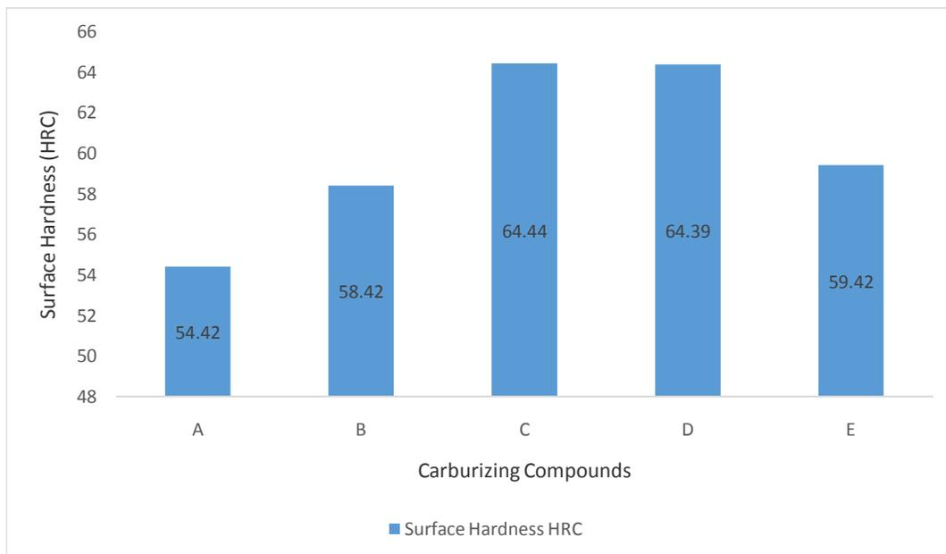
**Figure 8.** Bar chart of surface hardness variation with carburizing compounds.
