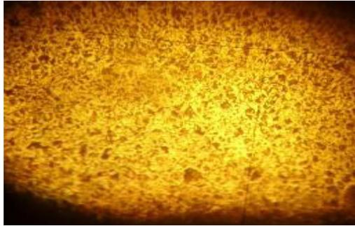
**Plate IV.** Micro structure of untreated mild steel with a pearlite structure in a ferritic matrix (Magnification X 200).
