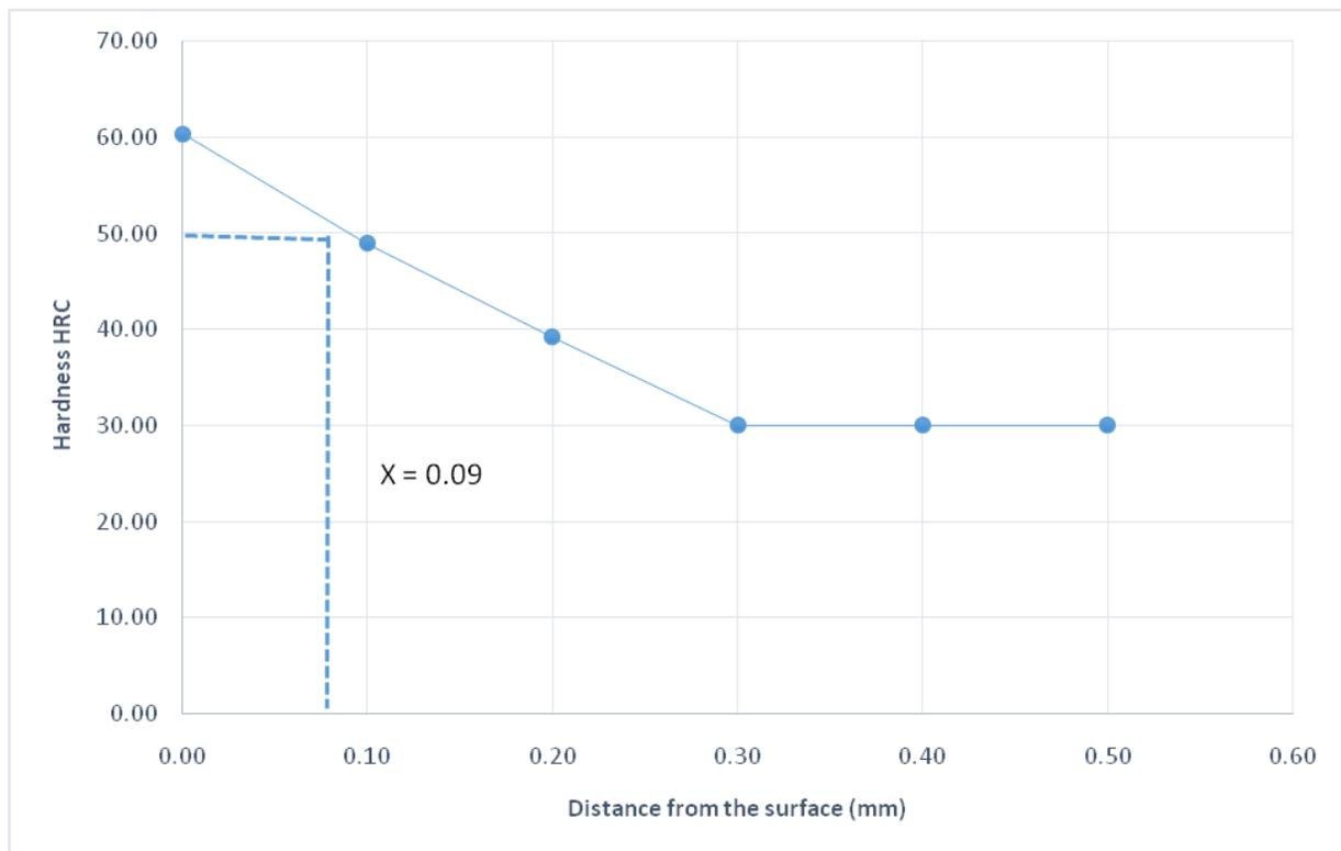
**Figure 4.** Hardness profile of carburized specimen using compound C against distance from the surface.
