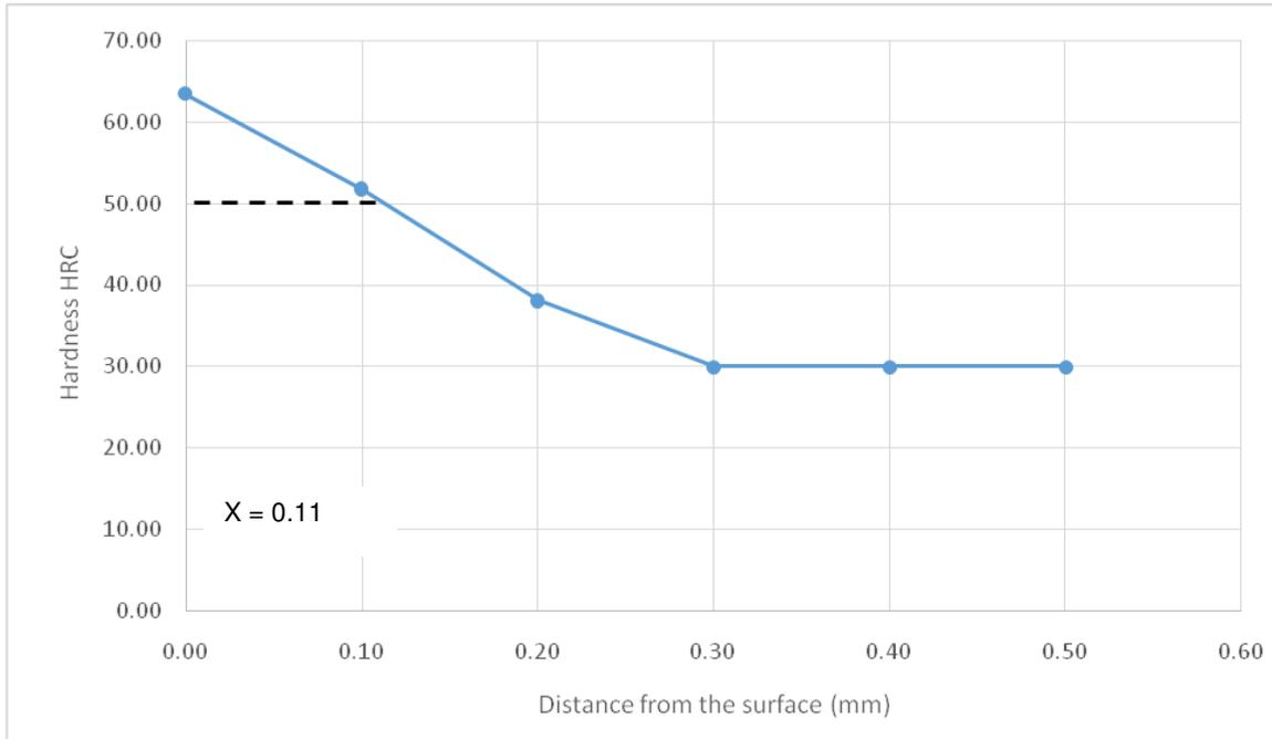
**Figure 5.** Hardness profile of carburized specimen using compound D against distance from the surface.
