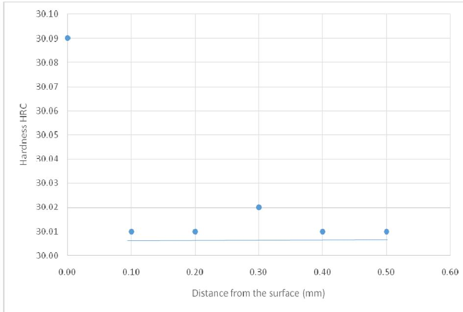
**Figure 1.** Hardness profile of un-carburized specimen against distance from the surface.
