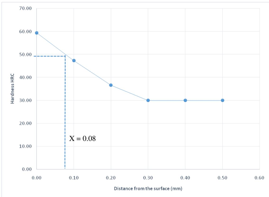
**Figure 6.** Hardness profile of carburized specimen using compound E against distance from the surface.
