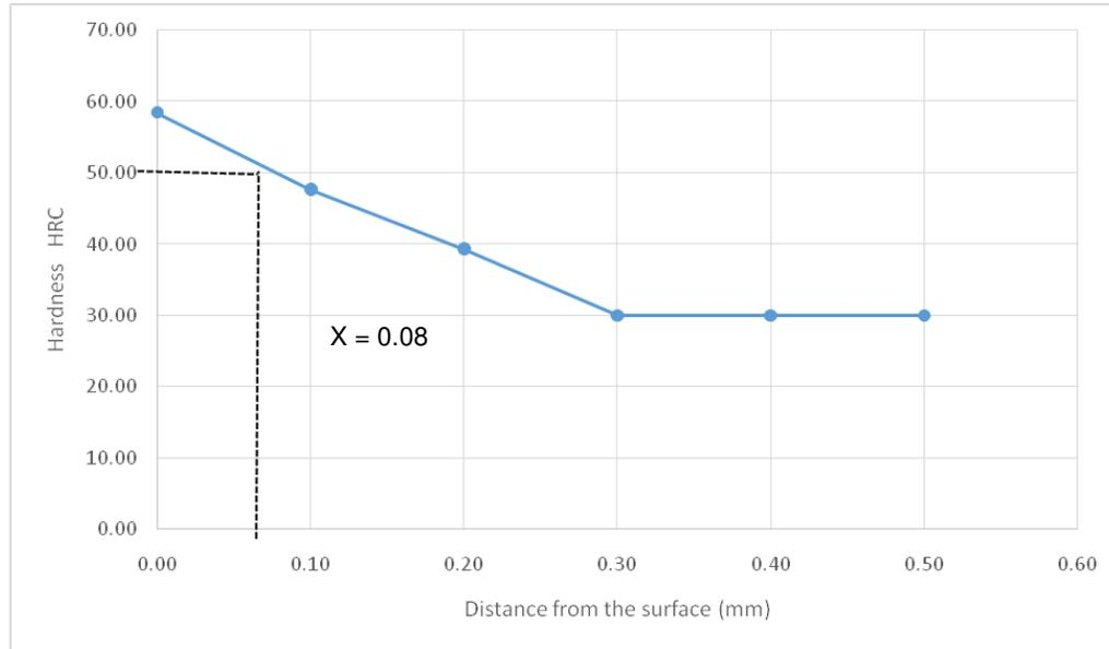
**Figure3.** Hardness profile of carburized specimen using compound B against distance from the surface.
