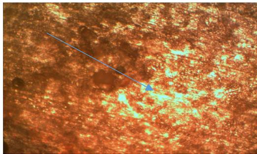
**Plate V:** Micro Structure of carburized specimen using compound D, showing Darker Case and Lighter Core (Magnification X 200).
