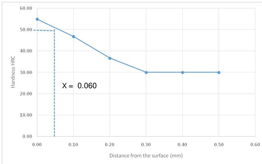
**Figure 2.** Hardness profile of carburized specimen using compound A against distance from the surface.
