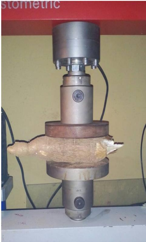
**Plate 1.** Cassava Tuber undergoing quasi compressive test using Universal Testing Machine (Testometric model).
