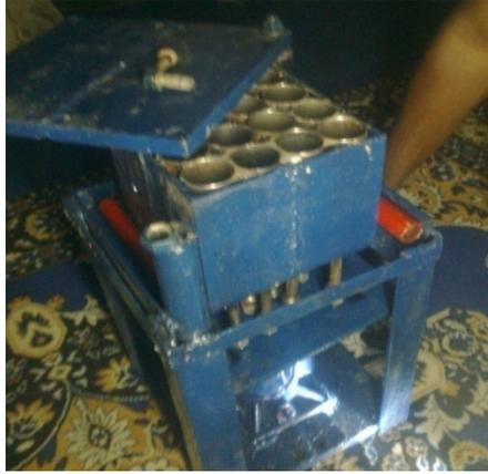
**Plate 1.** Fabricated hydraulic briquette making machine.
