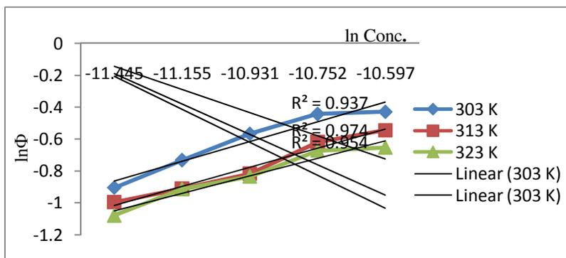
**Figure 6.** Freundlich adsorption isotherm of CFU on mild steel in 2M HCl at different temperature.
