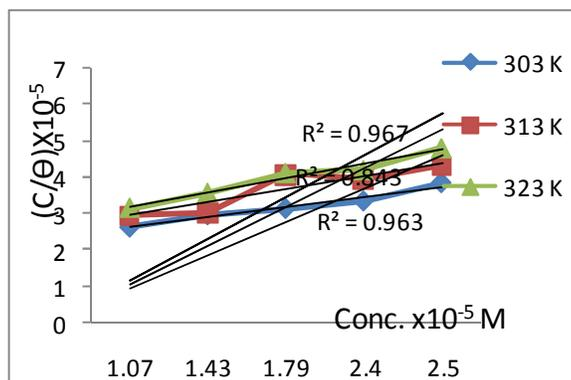
Figure 5. Langmuir adsorption isotherm of CFU on mild steel in 2M HCl at different temperature.
