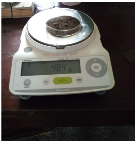
**Figure 1:** Taking the weight of the soil samples.
