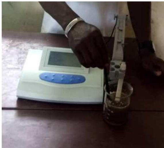
**Figure 2:** Determining the electrical conductivity of soil samples.
