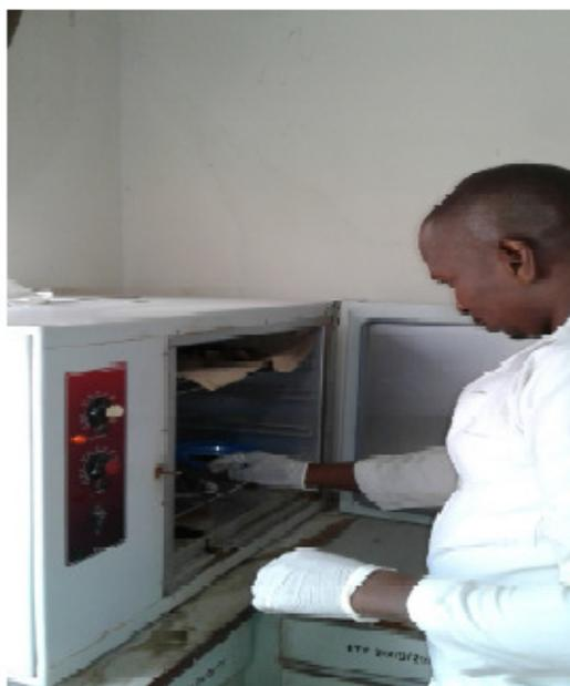
**Plate 4:** Drying of waste samples in an Oven at the laboratory as part preparations for samples analysis.
