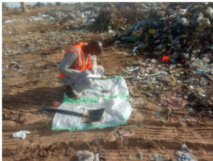
**Plate 3:** Taking coordinates of the sampling points using GPS at INEX Cleaners Dumpsite.
