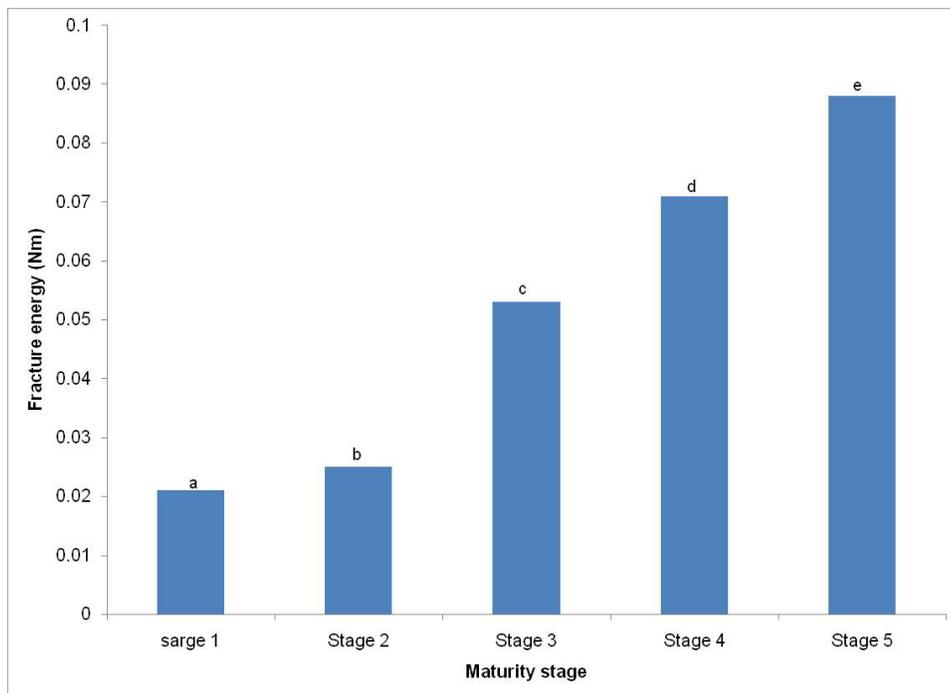
Figure 3: Fracture energy of okra seeds.
