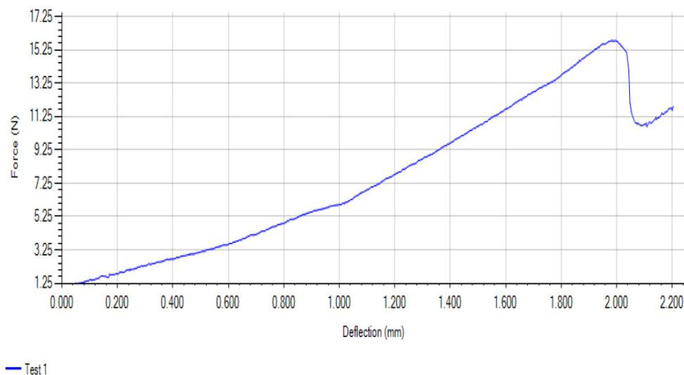
**Figure 1:** A force-deflection curve of the okra seed plotted by the machine.
