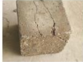
Figure 5: Cubes with intentional cracks
