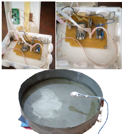
Figure 8: 3Dview of digital evaporation pan with logger.
